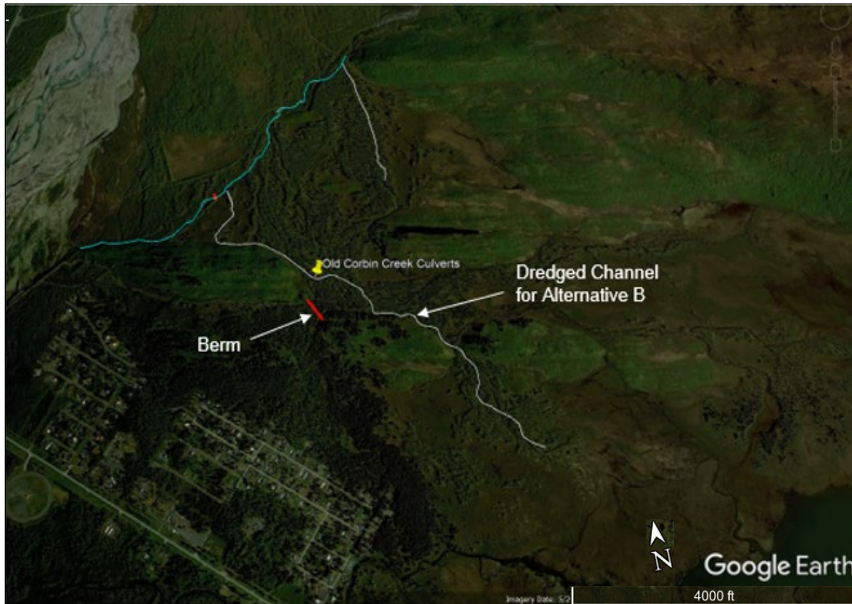
Figure 6-5. Alternative B: Excavated Channel Extents
